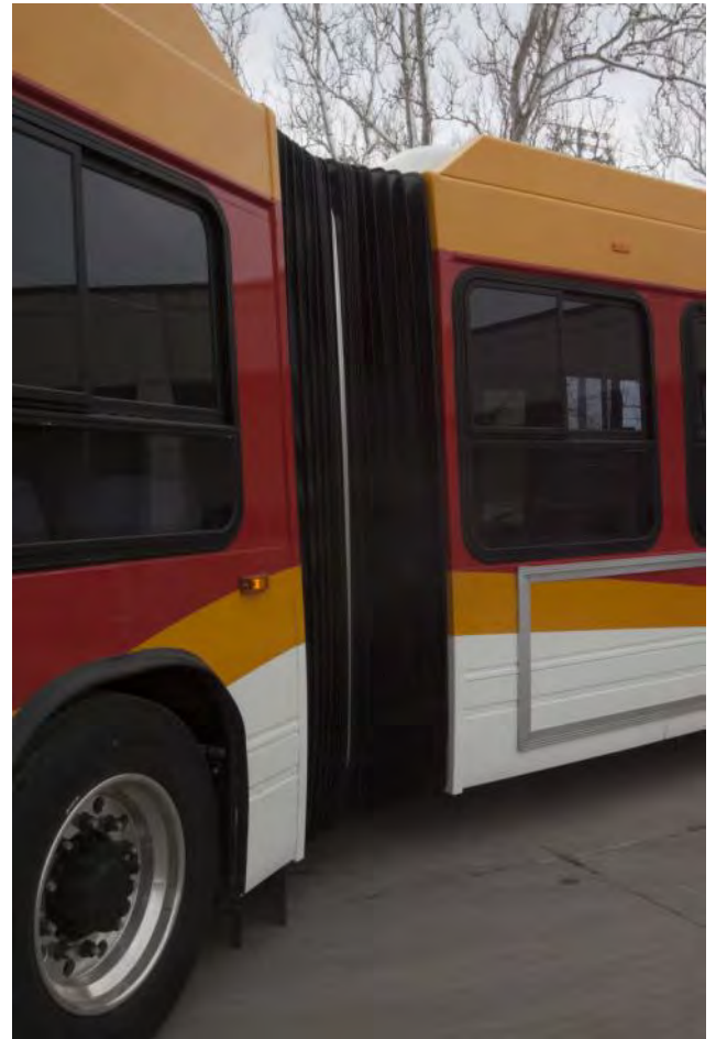
View – Outside View of Articulated Bus Turntable (the “bendy” part)
