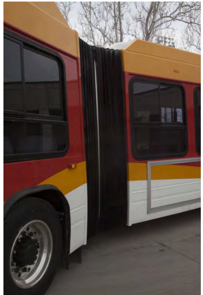
View – Outside View of Articulated Bus Turntable (the “bendy” part)
